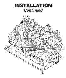
Figure 20 - Placement of Top Logs (Mossy Maple Logs Shown)
